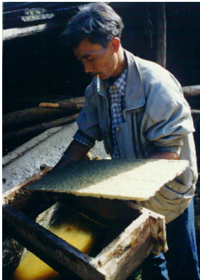
08 当纸浆均匀铺在模具底部的竹笪子上时，他缓缓提起模具，使水漏出，然后把铺满纸浆的竹笪子从模具中取出。 When the pulp is evenly distributed on the bamboo grate at the bottom of the mold, the mold is slowly lifted and the water runs out. The bamboo grate is taken out of the mold.
